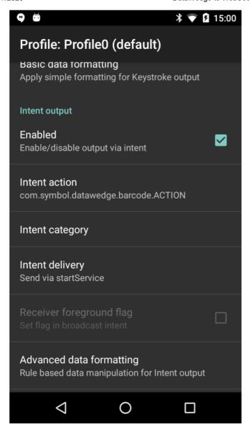
The above screenshot shows the Intent output portion of the DataWedge profile. Note we are sending Intents with the action 'com.symbol.datawedge.barcode.ACTION' and the default category.
